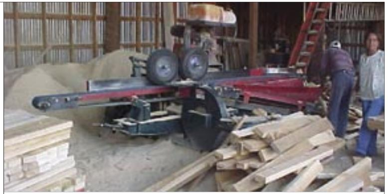
**Portable sawmill makes wood pallets out of small diameter material.**
