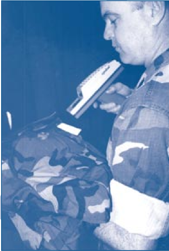
A Marine scans the bar code on an electronic "dog tag" attached to a battle dress uniform about to be issued. Data is stored in a computer system that tracks the transactions.
