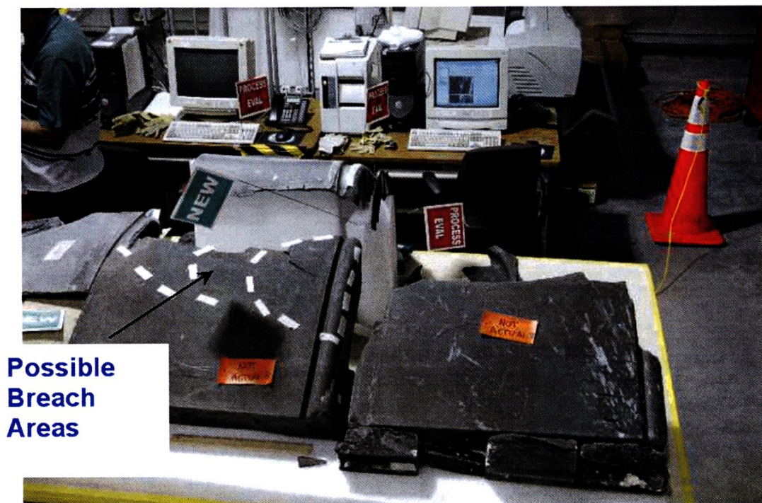
Figure 33: Probable Initial Breach in Panel 8.
