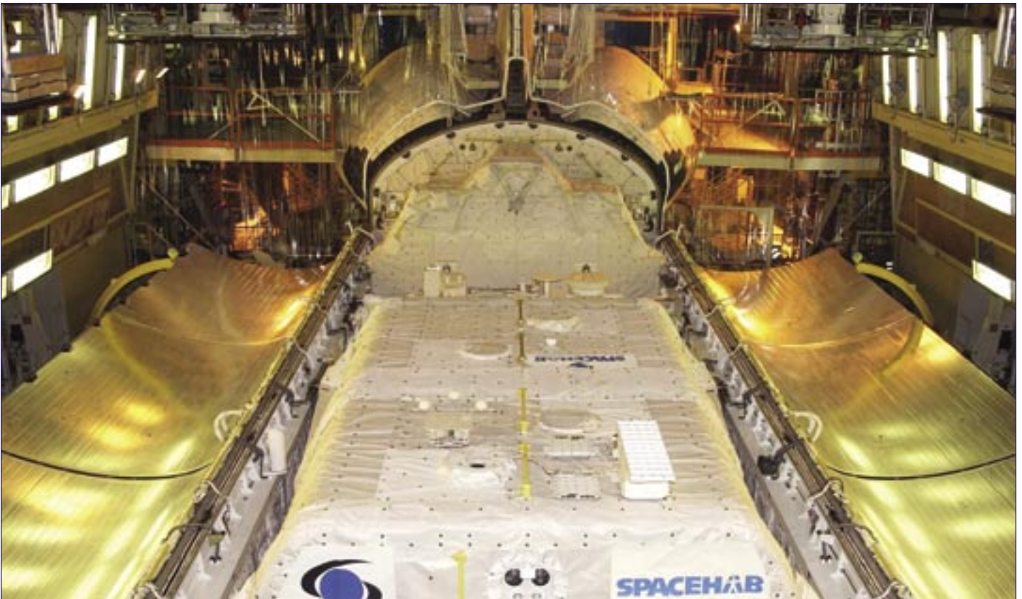
(Below) Columbia's payload bay doors are ready to be closed over the SPACEHAB Research Double Module on June 14, 2002.
