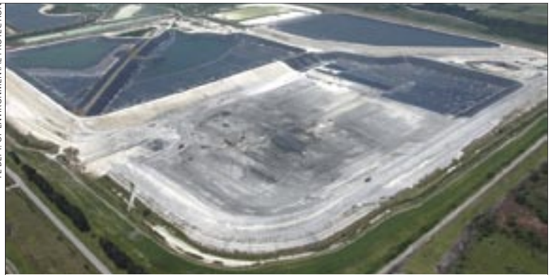
Three lined ponds and one partially lined pond are situated atop the Piney Point phosphogypsum stack ponds.
