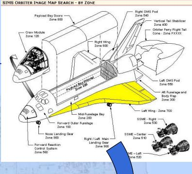
Inboard Elevon Left Wing Left Main Gear Wheel Well-Zone 751 Elevons & Zone 730 Wing/Elevon Interface Left Wing FWD Wing Box Zone 750 Left Wing FWD Wing Box -Leading Edge Left Wing Outboard Zone 752 Left Wing Leading Edge Left Wing Intermediate Box-Left Wing Torque Box Leading Edge Zone 720 Left Wing Intermediate Leading Edge Left Main Landing Gear, Door & Wheel Well (Ref.) Left Wing Bottom External Zone 910, 943, 730
