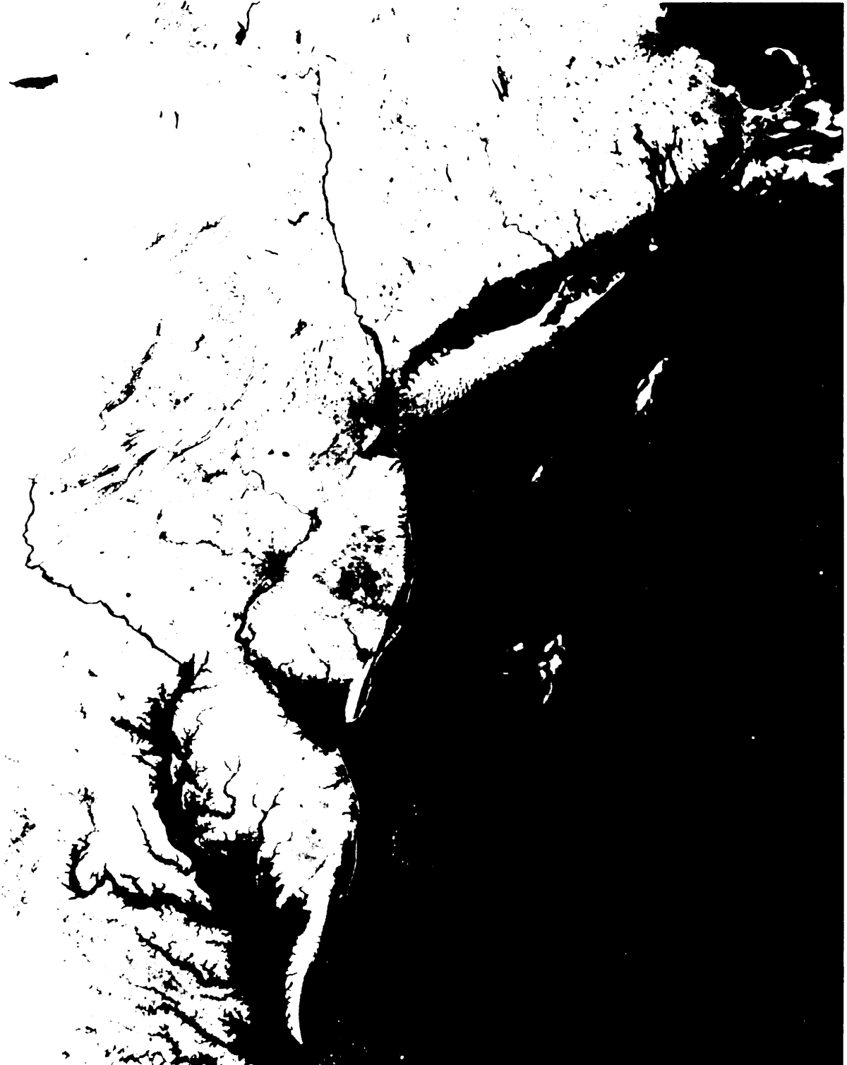
Figure 15.—A black and white copy of a color photograph taken by ERTS-1 of the area between Boston, Massachusetts and Norfolk, Virginia. The original color photograph contained 3 colors: bright red—depicting healthy crops, trees, and vegetation; industrial areas show up green or dark gray; clear water as black; suburban areas in light pink; and barren lands as light gray. NASA photo
