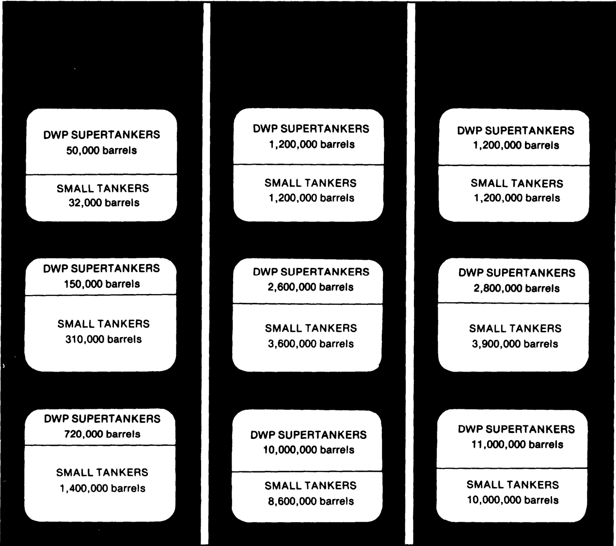
Figure IV-43. Fifteen (15) year totals of oil spills from one 1.6 million barrel per day deepwater port compared to small tanker alternative
