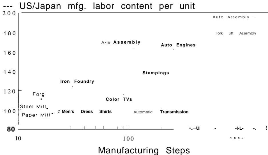
NOTE: As the number of steps in manufacture increases, the ratio of total factory labor content per unit of output of U.S. factories increases relative to Japanese factories,
